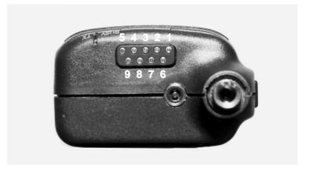
Figure 3.7 T3000 Accessory Connector - Top View
