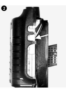
3 Fit the top of the rear cover assembly into the top of the front panel assembly, as shown. Check that the main seal remains correctly positioned on the shield.
