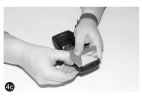
5 Remove the shim when the main seal is completely under the shield, and is not visible.
